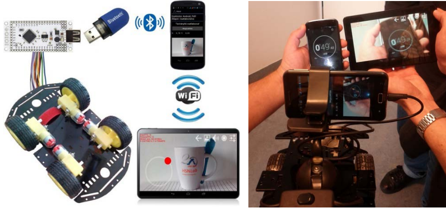
Figure 3: a) The elements of the mobile node and b) the implemented vehicle.
