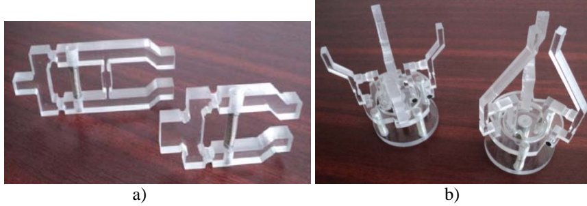
Figure 8: Compliant grippers: a) Normal and reverse actuating grippers b) Gripper with three and four fingers.
