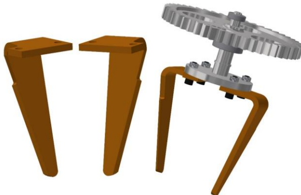
Figure 1: The solid models of the tines (left) and a working unit with two tines (right)
