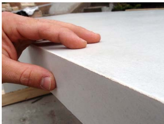
Photo 6: A UHPC bench's edge after being put in formwork, before being chamfered.
