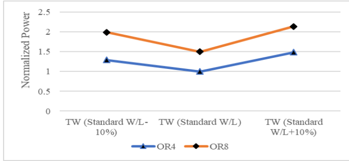
Figure 9: Power consumption for various W/L ratios of transistor Tw
