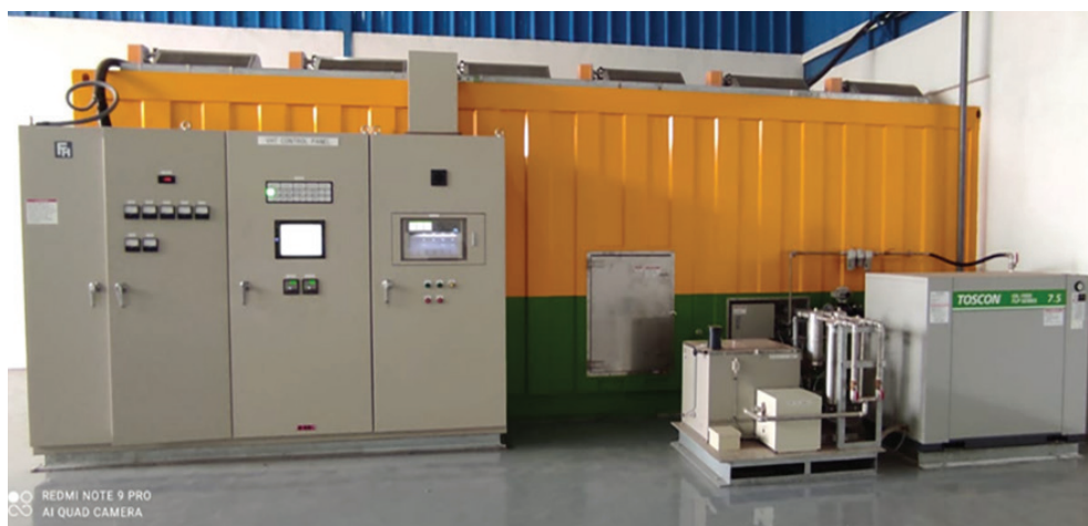
Figure 6. Commercial-scale vapour heat treatment (VHT) machine in Indonesia (PT Buah Angkasa)
