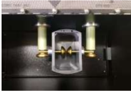
Figure 1: Electrode placement and shape in the DTS-60D
